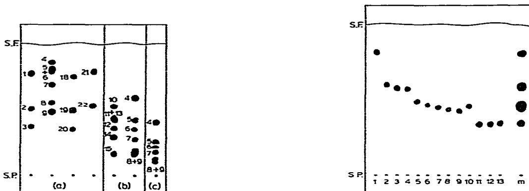
Fig. 1. Thin-layer chromatograms of halogenated phenols under different experimental conditions. Migration distance = 7 cm. The numbers refer to the compounds in Table I. (a) RP-18 + 4% HDBS plate with 1 M ammonia in 40% methanol as eluent; (b) RP-18 + 4% HDBS plate with 0.1 M ammonia + 0.1 M ammonium chloride in 60% methanol as eluent; (c) OPTI-UP C_{12} plate with 0.1 M ammonia + 0.1 M ammonium chloride in 20% methanol as eluent. S.P. = Starting point; S.F. = solvent front.
